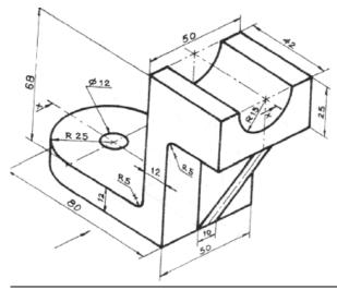
b) Draw the isometric view of the object, the orthographic views of which are 07 shown in the figure below.
